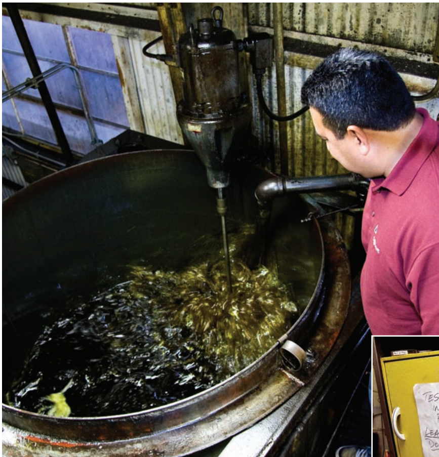
Oil being blended at Dodge Oil (above). The company's simple six-month oven test (right) helped set a baseline for VOCs in metalworking fluids.
